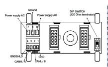
In case of Z-PC-DINAL-2-17,5 accessory, the signals may be provided by terminal blocks. The figure shows the meaning of the terminals and the position of the DIP-switch (present on each DIN rail supports listed on Accessories) for network termination (not used in case of Modbus network). GNDSHLD: Shield to protect the connection cables (recommended).
