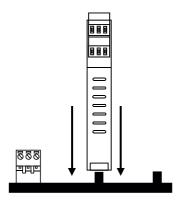
As it is illustrated in the next figure: 1) Insert the rear IDC10 connector on a DIN rail free slot (the inserting is univocal since the connectors are polarized).
