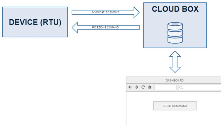
The devices don't just send data to Cloud BOX, but also alarm messages, which are asynchronous in relation to the sampling time, and arrive when they occur, rather than during the next data upload window (polling). During each connection, Cloud BOX can send commands to the device based on the needs of the user and how the dashboard was programmed.
