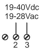
Power voltage must be in a range from 19 to 40 Vdc (indifferent polarity), from 19 to 28 Vac; see also section *INSTALLATION NORMS*.
