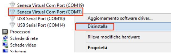
Now the COM3 is free and we can use it on the com0com setup:
