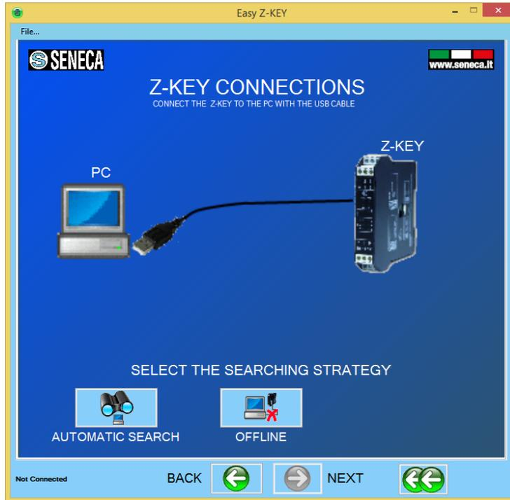
Then click on “Automatic Search”, read the configuration from the Z-KEY than modify the actual configuration with the new parameters:
