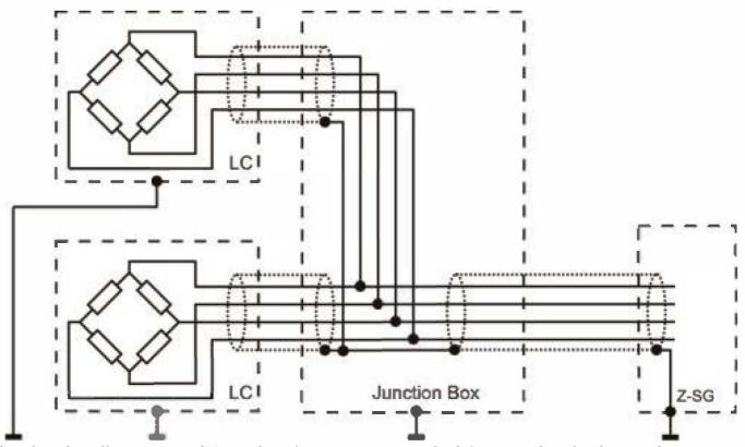
The load cell case and junction box are grounded by mechanical attachment to the structure to which they are mounted. Usually this structure is grounded.
