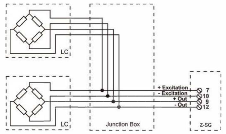
**6-Wire Load Cells Connections**
