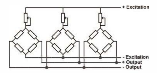
There are two methods of trimming with excitation. The first method is to adjust the potentiometers by trial and error whilst moving calibration weights around from corner to corner. All potentiometers should be adjusted to have the maximum sensitivity for each cell by completely turning clockwise all them.
