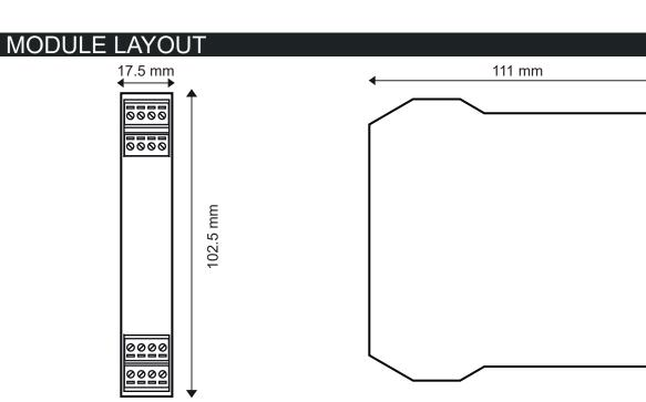
Dimensions LxHxD 17.5 x 102.5 x 111 mm; Weight: 110 g; Enclosure: PA6, black SIGNALS VIA LED ON FRONT PANEL
