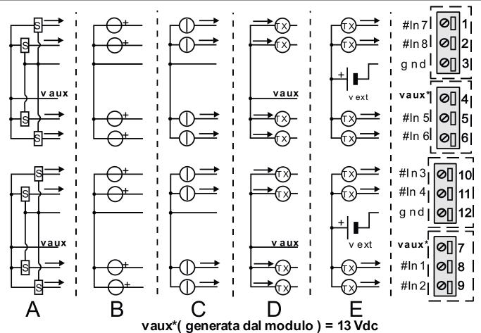
A) Voltage input with sensor supply from the MODULE (13 Vdc)
