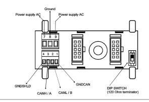
In case of Z-PC-DINAL2-17.5 / Z-PC-DINAL1-35 accessory use, the signals may be provided by terminal blocks. The figure shows the meaning of the terminals and the position of the DIP-switch (present on each DIN rail supports listed on *Accessories*) for CAN network termination. **GNDSHLD**: Shield to protect the connection cables (always recommended)
