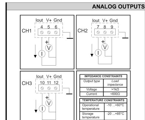
Every analog output has a 3-wires terminals:
