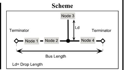
For the best performances, the use of special shielded cables is recommended (*BELDEN* 9841 cable for example).
