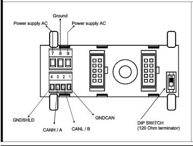
In case of Z-PC-DINAL1-35 / Z-PC-DINAL2-17.5 accessory use, the signals may be provided by terminal blocks. The figure shows the meaning of the terminals and the position of the DIP-switch (present on each DIN rail supports listed on *Accessories*) for CAN network termination. **GNDSHLD**: Shield to protect the connection cables (always recommended).
