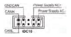
In the figure the meaning of the IDC10 connector pins is showed, in the case the user decides to provide the signals directly through it.
