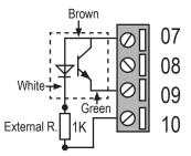
The internal power supply for the sensors, equal to 17 Vdc, is available at terminals 7 (+) and 10 (-).
