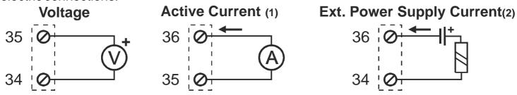
There is no insulation between RS485 and the analog output.
