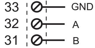
There is no insulation between RS485 and the analog output
