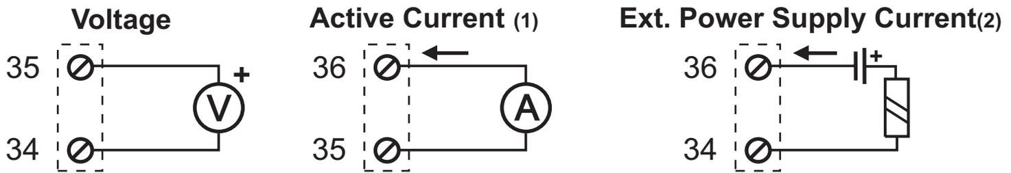
There is no insulation between RS485 and the analog output.
