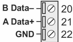
One RS485 serial port, for communication with the Modbus Master system, is available from terminals 20 – 21 - 22.
