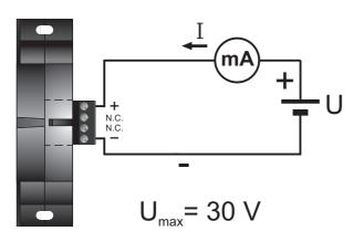
A maximum voltage supply of 30 V can be connected directly to the loop 4 – 20 mA of the T201DC100, extend up to 100 V the voltage supply with an external resistor as explained in the following page.
