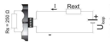
Supply voltage in the current output loop can be extended up to 100 V. Using an external resistor in series with T201DC100, in order to dissipate excess power supply. Consider the circuit shown on the left to calculate the value of Rext.
