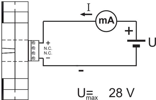
It is possible to connect directly on the 4 ÷ 20 mA loop in T201DC100 output a maximum voltage of 28 V.
