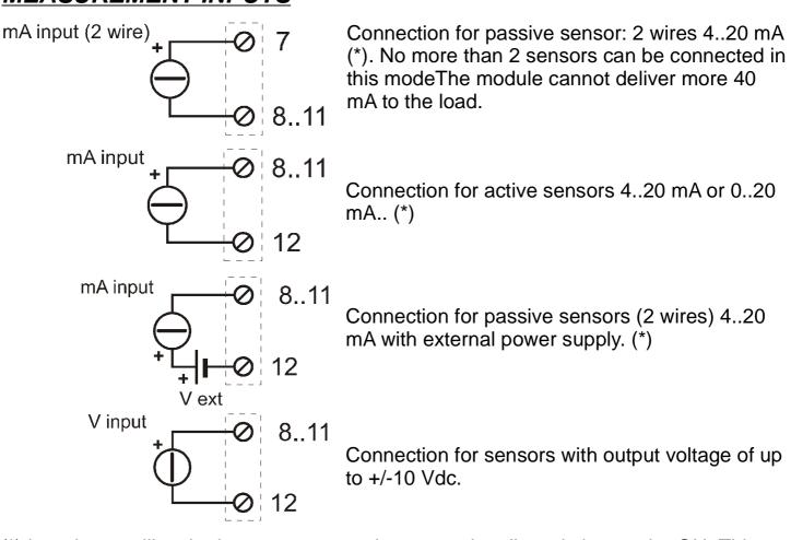
(\*) in order to utilise the input as current, the respective dip-switch must be ON. This operation connects a 100 Ohm resistance parallel to the input terminals and permits a signal of +/- 2000 mV to be obtained near +/- 20 mA.
