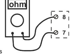
Example: if the reading is 30,000 ohm, the full-scale value is increased by 30,000 / 2,.000 = 15 V
