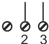
Power supply voltage must be in the range 9..40 V<sub>DC</sub> (at any polarity), 19..28 V<sub>AC</sub>; also see section; **INSTALLATION INSTRUCTIONS**.
