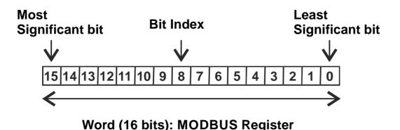
The Bit notation [x:y] shown in the table indicates all the bits from x to y. For example, Bit [2:1] indicates bit 2 and bit 1, and illustrates the meaning of the various linked combinations of the values of the two bits. Remember that the MODBUS 3 and 6 functions (respectively of multiple reading and single writing) can be executed on the following registers. Default values are marked with \* symbol.
