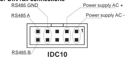
There is no isolation between RS485 and the retransmitted output.
