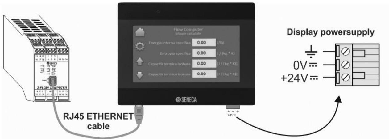
For correct operation, the first three values of the IP address of the screen must be the same as those of Z-FC, while the last value will be different.
