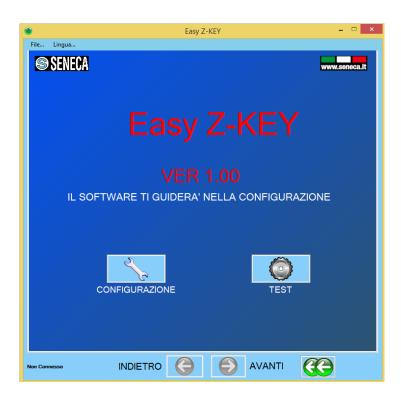
Connect Z-KEY to a PC with a standard micro USB cable, power up the Z-KEY and Click on "TEST" to obtain the actual IP address:
