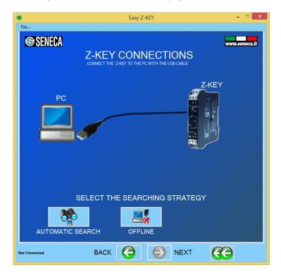
Than click on "Automatic Search", read the configuration from the Z-KEY than modify the actual configuration with the new parameters:
