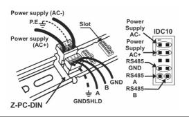
In the figure you can see the meaning of the IDC10 connector pins if you want to provide signals through them.
