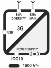
1500 V ∼ insulation between modem and power supply
