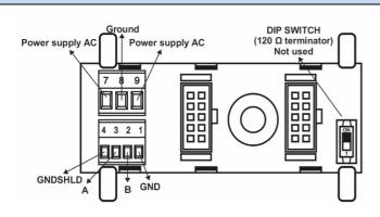
If the Z-PC-DINAL1-17.5 accessory is used the power supply
