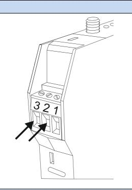
The power supply must be connected to the IDC10 bus or to terminals 2 and 3.
