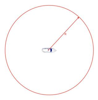
An alarm is generate if the vehicle is moved and exits the virtual fence:
