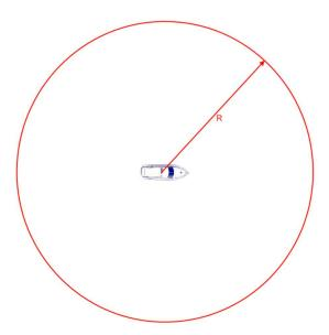
An alarm is generate if the vehicle is moved and exits the virtual origin:
