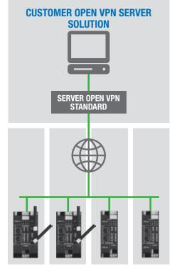
Client VPN (Z-PASS1/2) has to be installed. Telecontrol and Remote Assistance not supported
