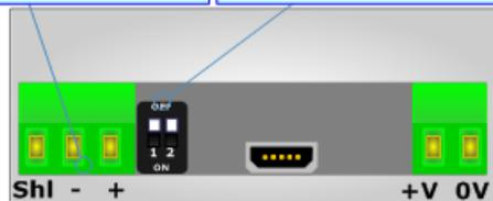
For terminate the RS485 line with a 220Ω resistor it is necessary that the 'Dip1' of the Dip-Switch B is at ON position.
