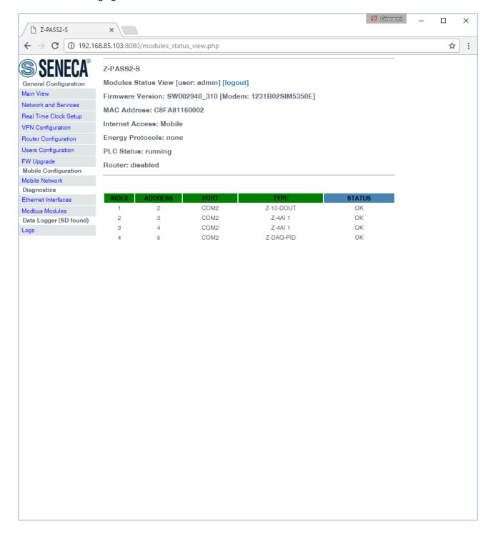
This page shows a table containing a row for each Modbus RTU Slave modules configured in the Z-NET4<sup>23</sup>/Straton project; each row contains the following information:
