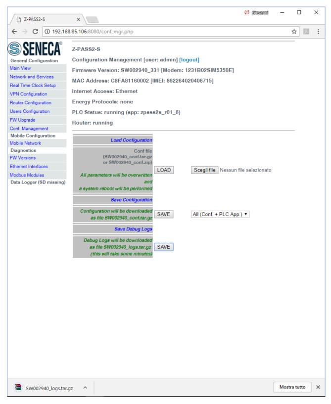
Please note that, to get detailed debug logs, the "DEBUG LOGS / Enable" parameter, in "Network and Services" page, shall be set to ON.
