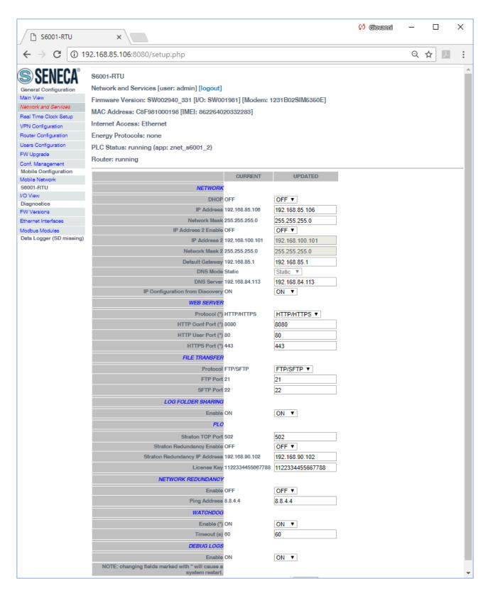
The previous figure shows the "Network and Services" page for a S6001-RTU; it also applies to a Z-TWS4 and Z-PASS2-S (old version).
