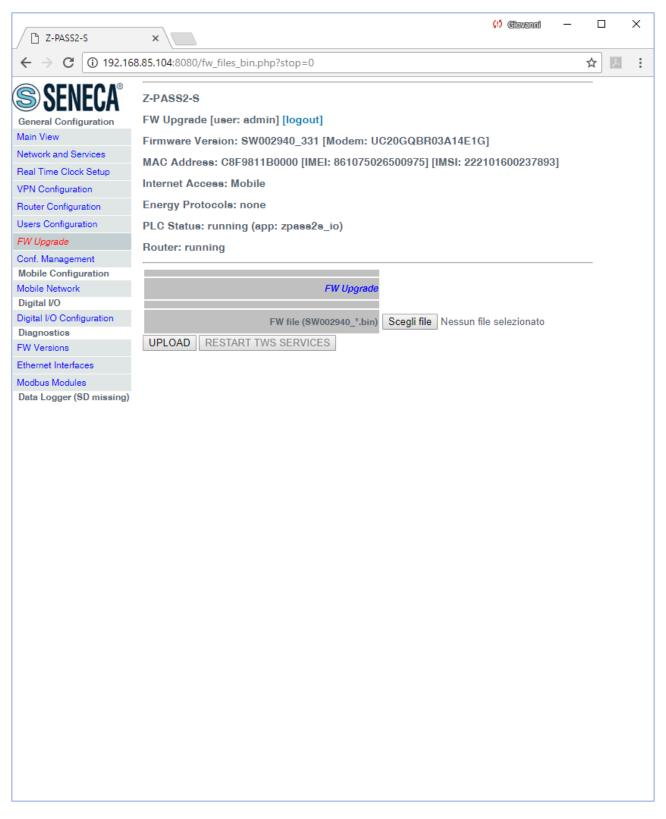
So, it is up to the user to choose if Soft PLC shall be stopped or not, during FW Upload; on one side, stopping it is more safe and let the upload be completed in a shorter time; on the other side, there are situations in which PLC stop time shall be as short as possible.
