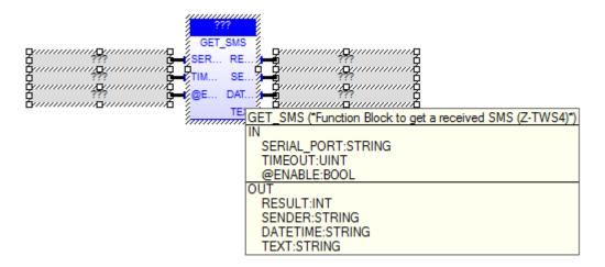
The GET\_SMS FB gets an SMS, previously received, by means of a GSM modem; once read, the SMS is deleted.
