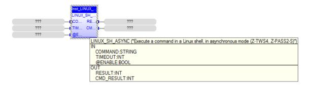
The LINUX\_SH\_ASYNC FB executes a command in a Linux shell, in asynchronous mode.
