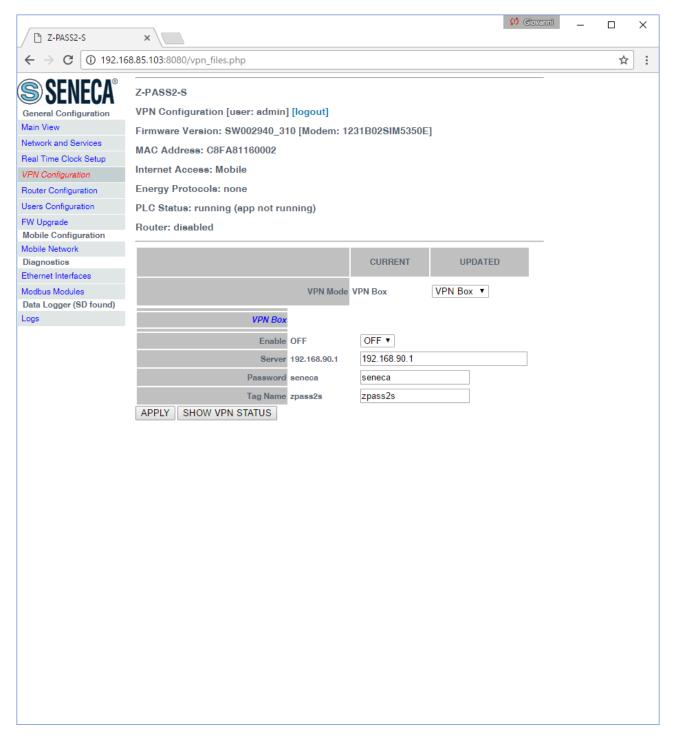
The page has a different layout depending on the value of the "VPN Mode" parameter, which can be "OpenVPN" or "VPN Box" (for an explanation of these values, see chapter 10).
