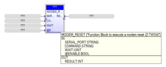
The  ${\tt MODEM\_RESET}$  FB sends an AT reset command to the GSM modem and waits for a specified time.
