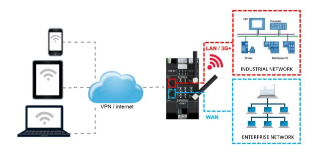
When this separation is not needed or when the Internet access is achieved only through the mobile (3G+) interface, the "Switch" mode still lets the Device be used as an Ethernet switch, as shown in the following figure.
