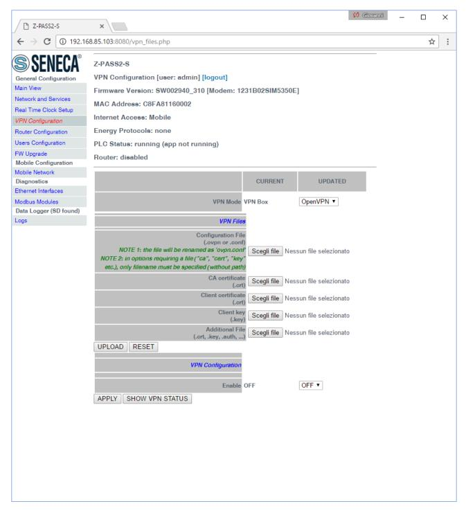
The "VPN Files" section lets you load the files needed to configure Open VPN and establish a secure VPN connection; these files are described in the following.
