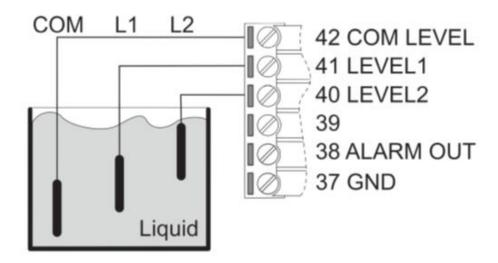
The analog level signals from screw terminals 40, 41, 42 can be used to control the level of liquid in a tank.
