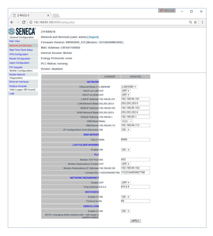
The previous figure shows the "Network and Services" page for a Z-PASS2-S-R01, when the "Ethernet Mode" parameter is set to "LAN/WAN"; it also applies to a Z-TWS4-R01 in "LAN/WAN" mode.
