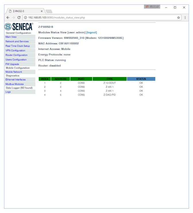
This page shows a table containing a row for each Modbus RTU Slave modules configured in the Z-NET4<sup>20</sup>/Straton project; each row contains the following information:
