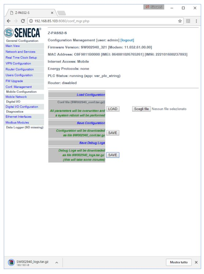
Please note that, to get detailed debug logs, the "DEBUG LOGS / Enable" parameter, in "Network and Services" page, shall be set to ON.
