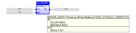
This FB permits to control the power ON/OFF digital input of the MODEM.
