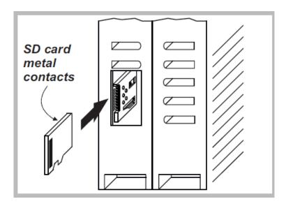
The Z-PASS2-S has a slot for SIM card, placed on the side of the case. Before pushing the SIM card into this slot, please be sure that the SIM card golden contacts are facing towards right (please see the figure below).
