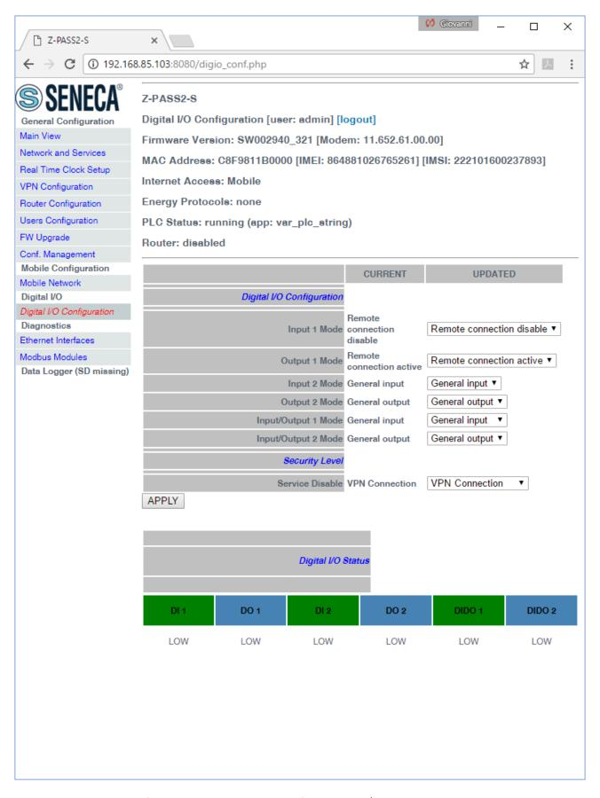
In this page, you can configure the operating modes of the Digital I/Os and the security level applied by the "Remote Access Disable" feature (see chapter 13).
