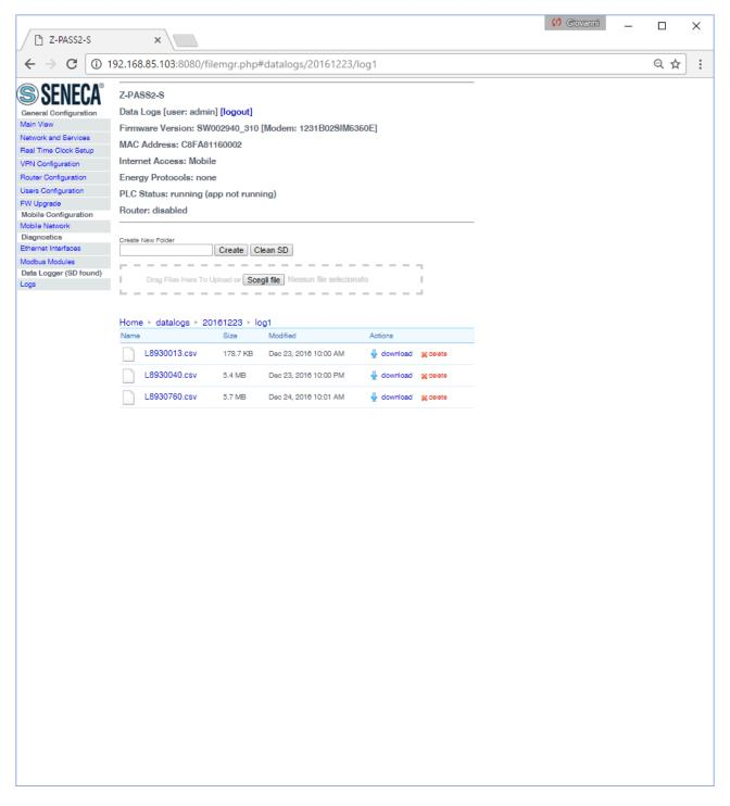
This page shows the contents of the SD card which, typically, is used to store "Data Logs" files; these files are created by the "Data Logger" functionality available in Z-NET4 "Remote Control Functions" (see chapter 18).
