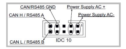
Power supply is available only from the rear connector for Z-TWS4, while Z-PASS2-S can be powered also through 14-15 screw terminals.
