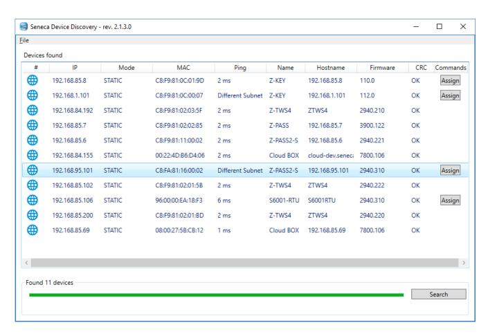
This application shows the IP address, MAC address, FW version and some other useful information, for every Z-TWS4/Z-PASS2-S/S6001-RTU device (and other Seneca products) found in the LAN.
