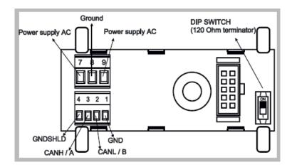
The Device has two RS 485 serial ports for Modbus communication: COM 4 and COM 2. The RS485 connection for COM 2 can be set up by means of the corresponding screw terminals or by the IDC10 connector. On Z-TWS4, to select RS 485 on IDC10 connector, put the SW1 DIP-switch on OFF position; on Z-PASS2-S, no operation is needed.
