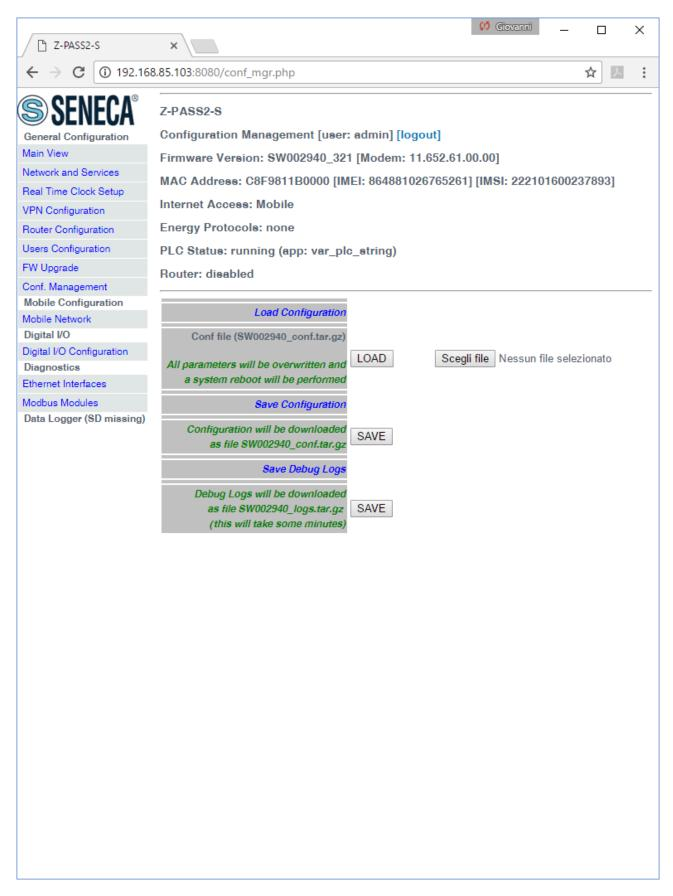
This page lets you save and load the whole Device configuration; this is very useful, for example, when you have to apply the same configuration to many devices.
