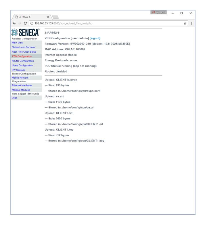
You can check which VPN files are stored on the Device by clicking on the "SHOW VPN STATUS" button, as shown in the following figure (remember that the configuration file is renamed as "ovpn.conf"):
