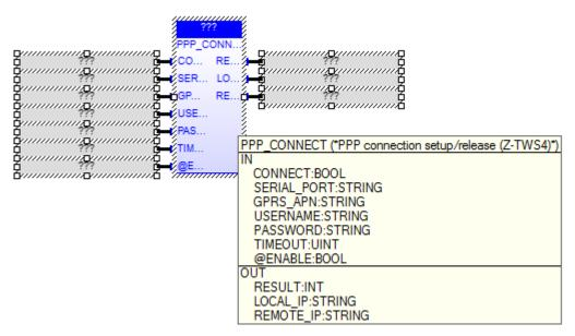
The PPP\_CONNECT FB performs PPP connection setup or release, by means of a  ${\tt GPRS/UMTS}$  modem.
