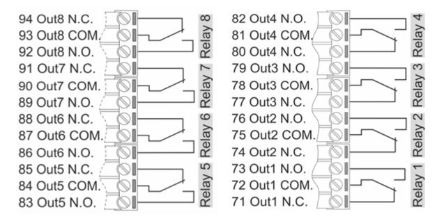
Eight SPDT relays are available to control, for example, external pumps. The operating voltage is 250 Vdc @ 2 A.
