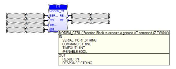
The MODEM\_CTRL FB sends a generic AT command to the GSM modem and receives the corresponding response.
