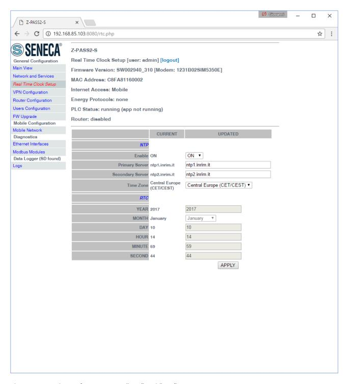
This page is made up of two sections: "NTP" and "RTC".
