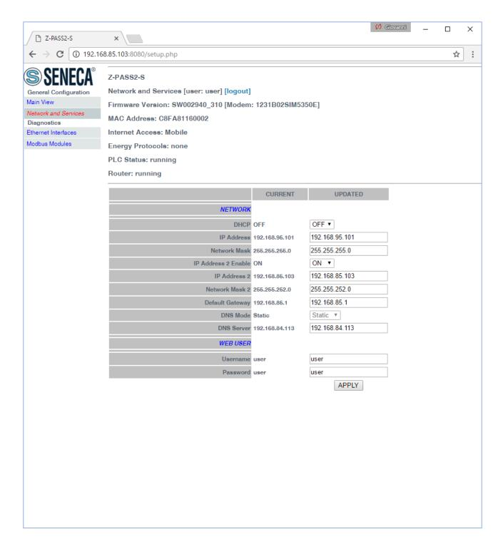
The previous figure shows the "Network and Services" page for a Z-PASS2-S-R01/Z-PASS2-S-R02, when the "Ethernet Mode" parameter is set to "Switch"; it also applies to a Z-TWS4-R01/Z-TWS4-R02 in "Switch" mode, to a Z-TWS4 and Z-PASS2-S (old versions) and to a S6001-RTU.
