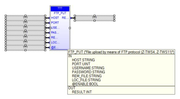
The FTP PUT FB uploads a file, by means of the FTP protocol.
