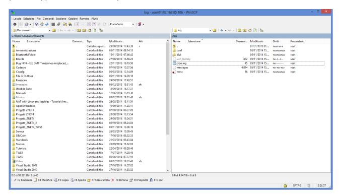
The WinSCP program can be used both as an FTP or SFTP client to transfer files to/from the Device; just select "FTP" or "SFTP" protocol in the "WinSCP Login" window; normally, it's better to use SFTP, since it provides a secure (i.e. encrypted) service.
