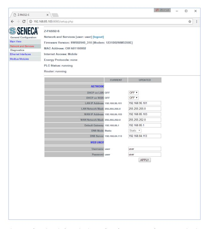
The previous figure shows the "Network and Services" page for a Z-PASS2-S-R01/Z-PASS2-S-R02, when the "Ethernet Mode" parameter is set to "LAN/WAN"; it also applies to a Z-TWS4-R01/Z-TWS4-R02 in "LAN/WAN" mode.
