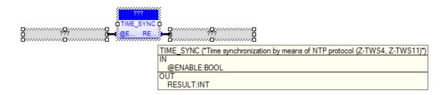
The TIME SYNC FB performs time synchronization, by means of the NTP protocol.
