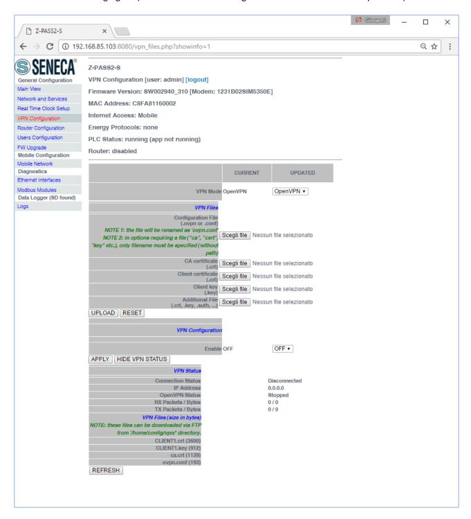
As reminded by the web page, the VPN files can be downloaded from the Device, if needed, via FTP/SFTP; they can be found in the /home/config/vpn directory, as shown in the following figure.
