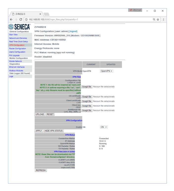
An important status information is given by the "OpenVPN Status" field; <u>if VPN is enabled ("ON")</u>, <u>but this status is "Stopped"</u>, <u>Open VPN process could not be correctly started: probably, the configuration file contains some errors or, maybe, some options not supported by the Device Open VPN implementation.</u>
