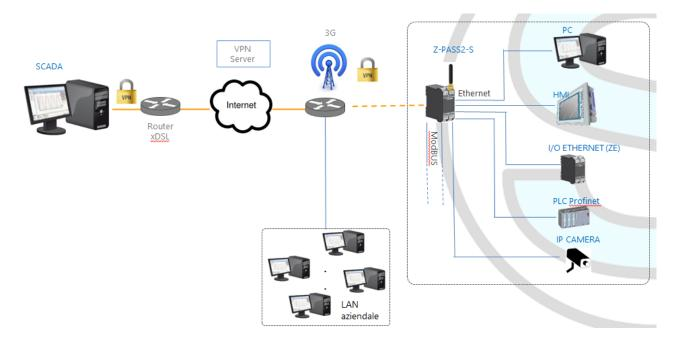
As already told before, "Router" functionality routes packets between the WAN (Mobile Network) interface and the LAN (Ethernet) interface and vice versa; so, this functionality especially makes sense when a 3G connection is active, which needs the availability of a 3G modem (always true for Z-PASS2-S and S6001-RTU, true for Z-TWS4 when connected to Seneca Z-MODEM-3G modem).
