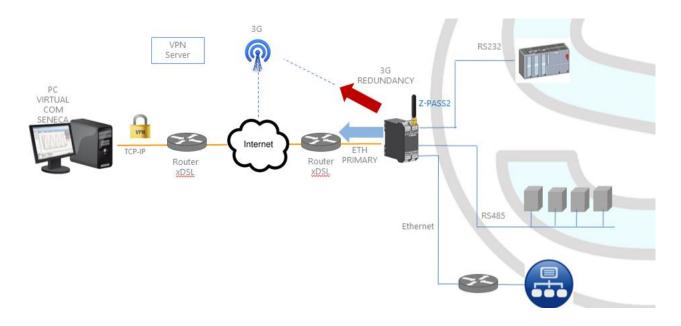
"Network Redundancy" is a functionality than can be enabled on the Device when a 3G modem is available (always true for Z-PASS2-S and S6001-RTU, true for Z-TWS4 when connected to Seneca Z-MODEM-3G modem).
