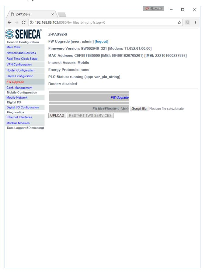
So, it is up to the user to choose if Soft PLC shall be stopped or not, during FW Upload; on one side, stopping it is more safe and let the upload be completed in a shorter time; on the other side, there are situations in which PLC stop time shall be as short as possible.
