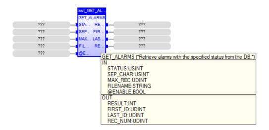
This FB retrieves all alarm records with the specified status from the DB; the records are written as lines into the specified file.
