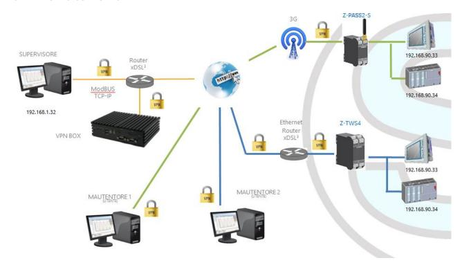
The above figure gives an example of a "Point-to-Point" VPN.
