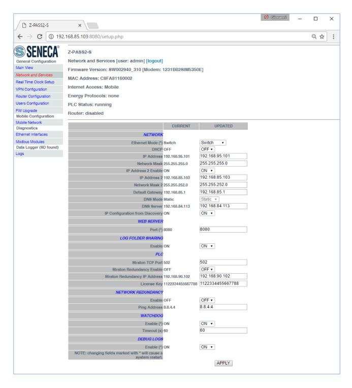
The previous figure shows the "Network and Services" page for a Z-PASS2-S-R01, when the "Ethernet Mode" parameter is set to "Switch"; it also applies to a Z-TWS4-R01 in "Switch" mode.
