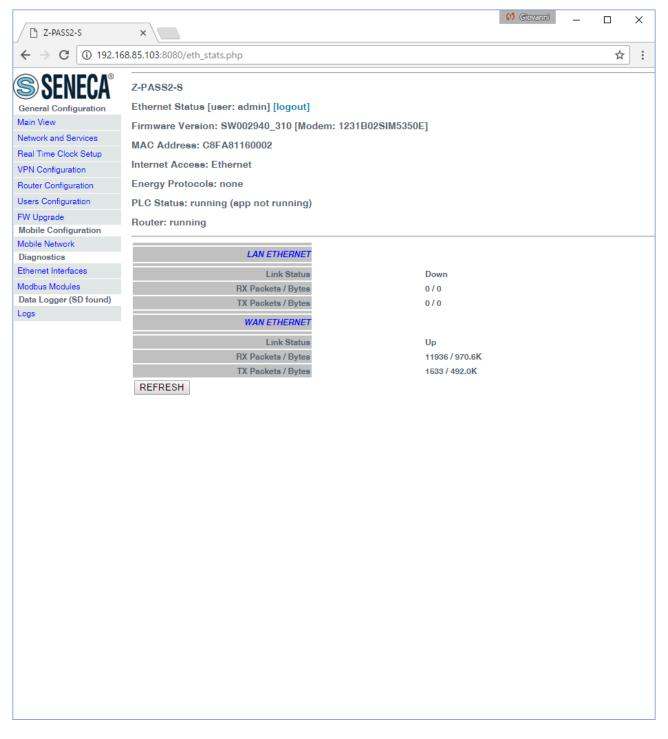
The above figure applies to a Z-PASS2-S-R01/Z-PASS2-S-R02 CPU, when the "Ethernet Mode" is "LAN/WAN"; a similar page also applies to a Z-TWS4-R01/Z-TWS4-R02 CPU.
