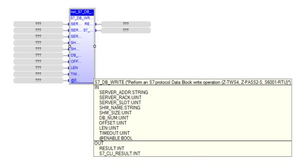
This FB performs an S7 protocol Data Block write operation.
