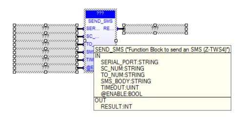
The SEND SMS FB sends an SMS, by means of a GSM modem.
