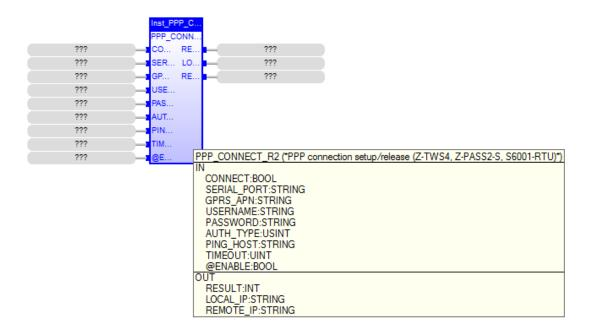
The PPP\_CONNECT\_R2 FB performs PPP connection setup or release, by means of a GPRS/UMTS modem.
