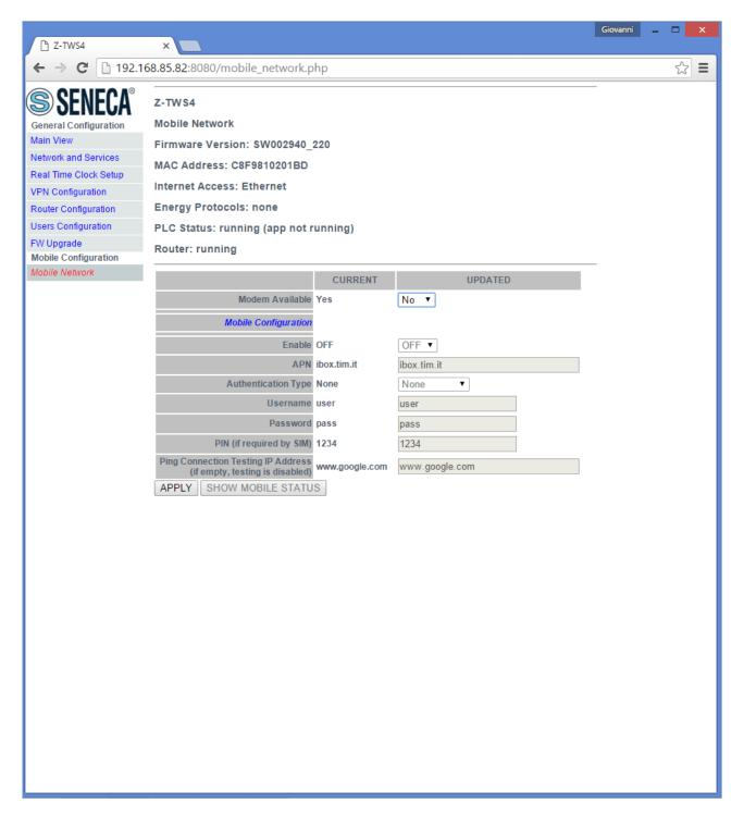
If "Modem Available" parameter value is changed, when clicking on the "APPLY" button the system is restarted, as shown in the following figure:
