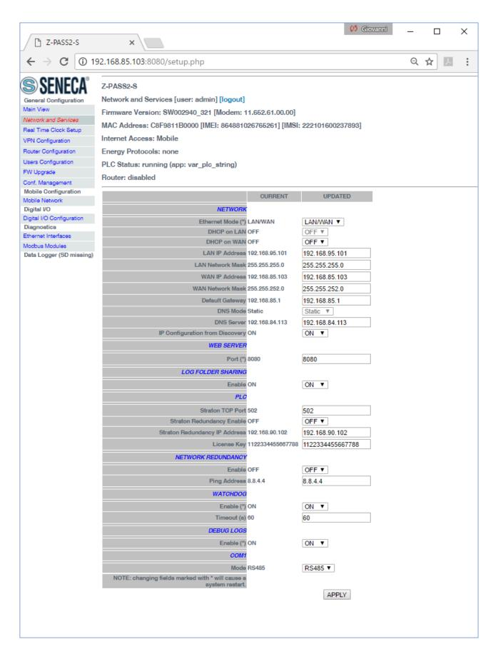
The previous figure shows the "Network and Services" page for a Z-PASS2-S-R02, when the "Ethernet Mode" parameter is set to "LAN/WAN"; it also applies to a Z-TWS4-R02 in "LAN/WAN" mode.
