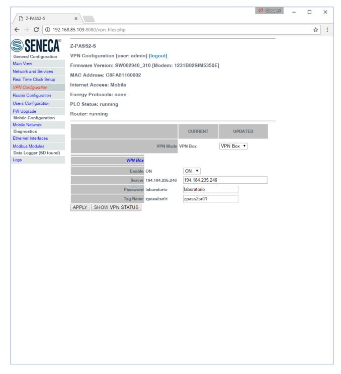
The "VPN Box" section contains the following parameters:
