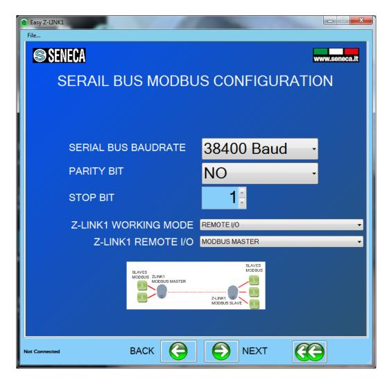
The Z-Link1 that act as Modbus Slave is called "Remote I/O Modbus Slave"
