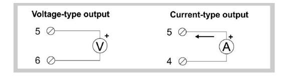
Shielded cables are recommended to connect the outputs (through screw terminals: 5, 6 if voltage-type output; 4, 5 if current-type output).
