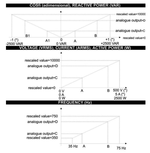
(\*) Limit values of voltage, current, cosfi depend on the dip-switch SW2-4,5. In the previous figures are shown the limits related to 100% retransmission scaling.
