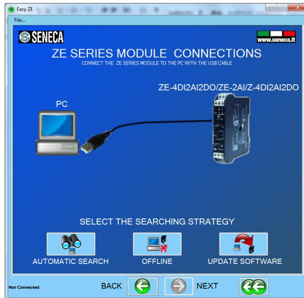
If you have previously installed the USB drivers connect the USB cable to the PC.
