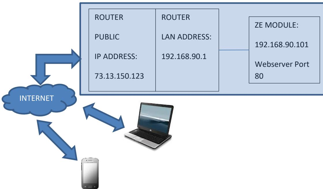
Now we must open the port 80 on the router and forwarding it to the IP 192.168.90.101:
