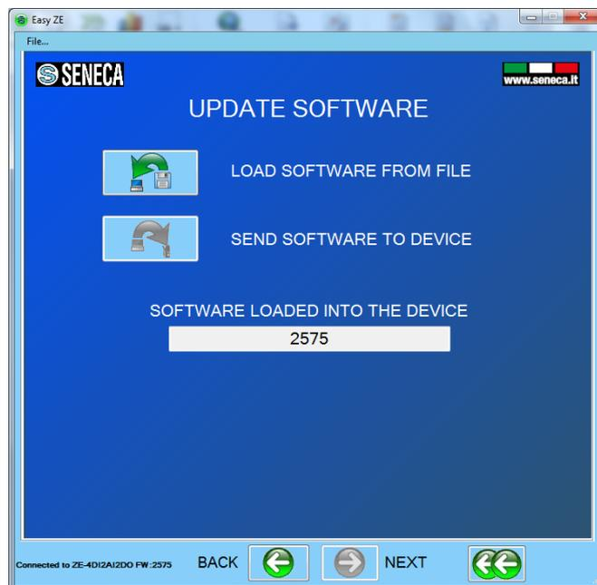
Press the "Load software from file", the software will open directly the firmware directory.
