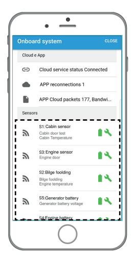
For a correct reading of the sensors dedicated to the control of the battery voltage and the voltage deriving from the platform (sensors S4, S5 and sensor inside the control unit identified as C1 in the user manual), it is necessary to manually modify the reading threshold.
