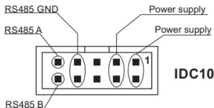
In the figure the meaning of the IDC10 connector pins is showed, in the case the user decides to provide the signals directly through it.
