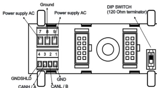
In case of Z-PC-DINAL-2-17,5 accessory, the signals may be provided by terminal blocks. The figure shows the meaning of the terminals and the position of the DIP-switch (present on each DIN rail supports listed on Accessories) for network termination (not used in case of Modbus network).
