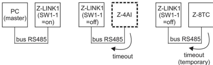
After a time interval of about 1 minute, the timeout message on the slave devices actually belonging to the network disappears, returning to the normal functioning. The behavior just described can be observed if there is the absence of the Z-LINK1 device connected to the interested Modbus slave device, too (for example, the previous Z-LINK1 connected to the Z-4AI via local bus).
