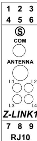
Devices directly involved in the transmission of messages may show the flashes on both L1 and L2, or only on L2. In the first case are terminal devices, while in the second case are intermediate devices, which have the only function of forwarding the packet via radio.
