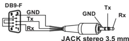
The module has a Jack stereo connector in order to connect its to RS232-bus communication. The frontal COM port is used to program the Z-LINK1 only.
