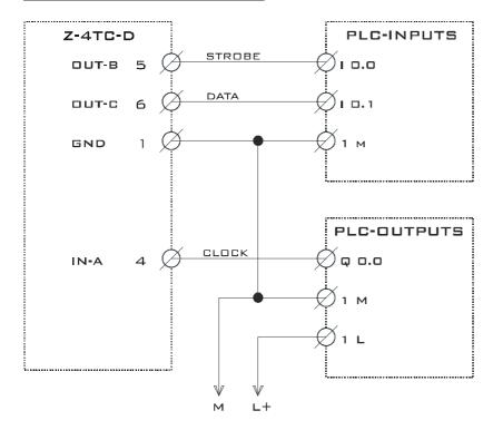
Although the connections indicated regard a SIEMENS S7-200 CPU 224-DC/DC/DC PLC in particular, other PLCs can also be used provided that their inputs are fast enough ( < 2 ms) and their outputs are transistor and not relay type.
