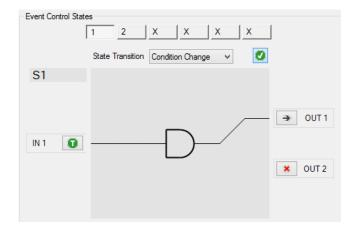
And the "IF (INPUT1 = FALSE) Then Execute Action Output 2" can be create din the State 2 (S2):
