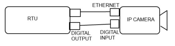
*IP Camera Folder:* Configure the RTU FTP Server where the IP camera will put videos and/or snapshots. When a new file is written in this folder the RTU will send the data from the Log notification channel configured (Ethernet or GPRS) to the profiles that includes the logs group. When a file is correctly sent the RTU will delete it from the local ftp.
