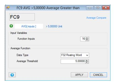
*Function Inputs:* Select the input pad numbers (from 2 to 16). Note that you can't leave unconnected an input pad.
