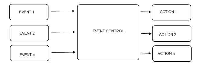
One or more *events* must be connected to an *event control*, this block performs the logic and select the right *action* output.
