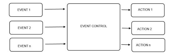
The EC inputs accept boolean events, each event control output must be connected to an action.
