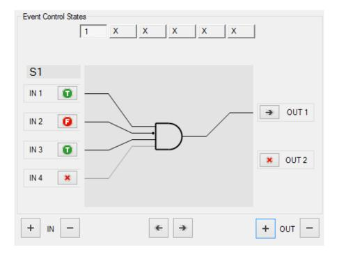
Then if the Digital input 2, 3 and 4 must be True for obtain a digital output 1 reset:
