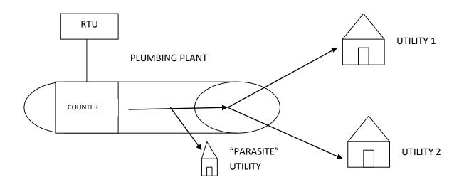
If this is not the case it means that there is a "parasite" utility in addition to the 2 utilities that continuously subtracts liquid (especially at night it is improbable that the utilities use water on all the 10 minute intervals).
