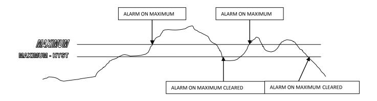
If the threshold is Minimum or Low the alarm is activated when the analog input is < threshold but the alarm rearm is obtained when at the analog input is > (Threshold+Hysteresis).
