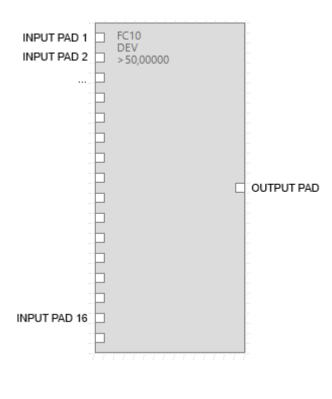
This block function calculate the absolute difference between an input and the average of all the inputs, than compare all this values with a threshold, if at least one of these compares is true the output is true too.
