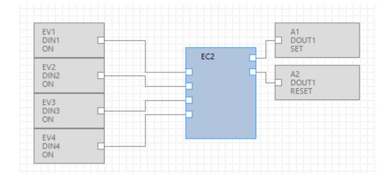
For example if we want to set the output1 if the Digital input 1 and 3 are True but the digital input 2 is false:
