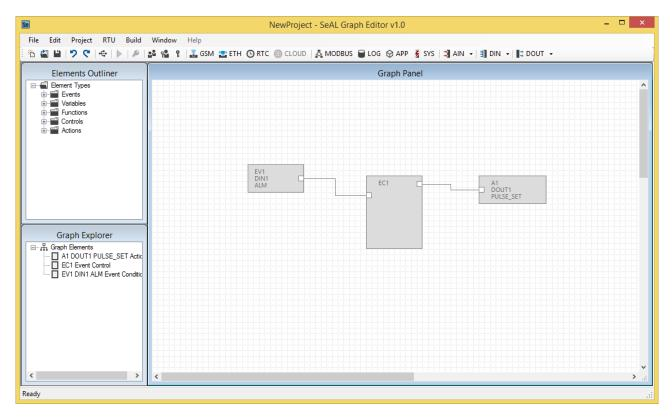
*The Element Outliner window* contains the database of blocks that are used into the Graph Panel window to build a program.
