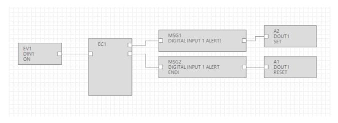
Configure the EC1 block for routing the alert condition in state S1 and the alert end condition in state S2:
