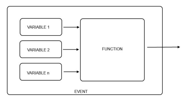
In SEAL a single event block is for example a Digital input alarm event:
