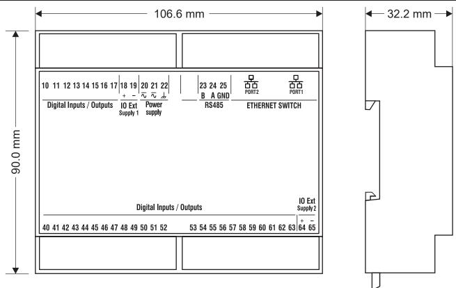
Weight: 170 g; Enclosure: UL94-V0 self-extinguishing PC/ABS material, black.
