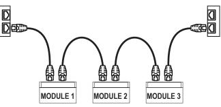
There must be no loops in the Ethernet cabling, otherwise the communication will not work. The modules and switches must be connected eliminating any loops. The following examples show the incorrect connections.
