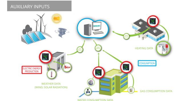
• MEASUREMENT OF WATER, HEAT, GAS ETC. CONSUMPTION VIA PULSE INPUTS
