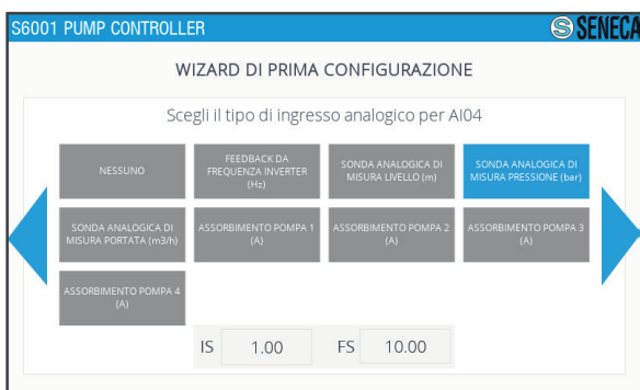
Fig. 25 Pressure/flow wizard - Type of AI04 analogue input
