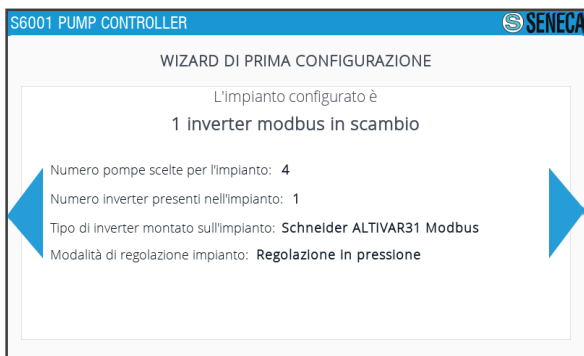
Fig. 23 Pressure/flow wizard - Inverter interface
