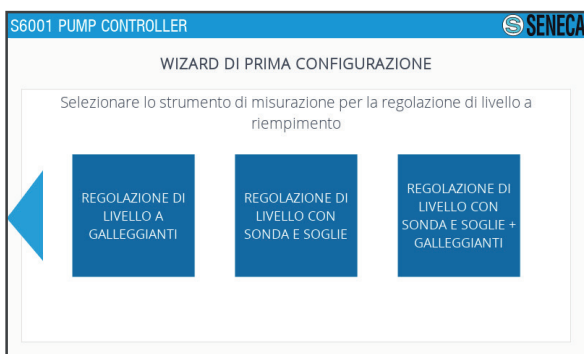
Fig. 33 Level wizard - Level adjustment applications
