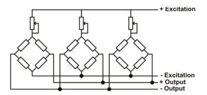
A variable resistor, independent of the temperature, or a typically 20  $\Omega$  potentiometer is inserted in the +Excitation cable of each load cell. There are two ways to trim the load cells. The first method is to adjust the potentiometers by trial, shifting the calibration weights from one corner to another. All the potentiometers must be adjusted so as to set the maximum sensitivity for each cell, turning them all completely clockwise. Then, once
