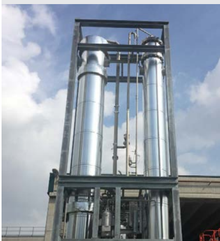
GM-GreenMethane Upgrading Unit with 125 m 3 /h biomethane
