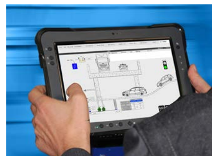
Synoptic monitoring of the underpass performed by Scada
