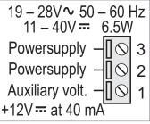
The power supply must be connected to terminals 2 and 3.
