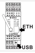
The module has a RJ45 socket on frontal panel.
