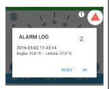
When the set threshold is exceeded, a flashing icon indicates that an alarm is present, or that the threshold has been exceeded. During this stage, if set to do so, your device will send a notification SMS to the recipients. The device will not send any further SMS until the alarm is "rearmed".
